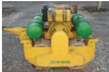
Compaction of wet granular base
